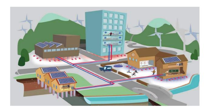
Sister manufacturing facility Centrum Pile has taken great steps to reduce its carbon footprint. After solar energy, geothermal energy is the second most abundant source of heat on earth. In this case, it is used in conjunction with Energy Piles, which are equipped with individual or several pipe circuits to enable the exchange of heat with the surrounding soil.
