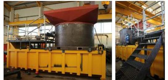
As we speak, we are currently building a dedicated portable grout mixing plant, complete with holding tank, for geotechnical projects. It has been designed in house and will be one of two to be built, with the first one expected to be completed in early January. We have also built a store for grout ash, providing a designated area on sites to avoid contamination and make it contained holding bin.
