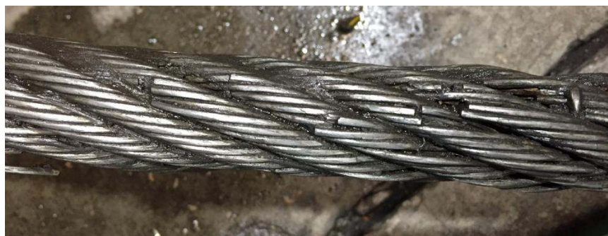
Cleaned rope showing multiple fatigue breaks
