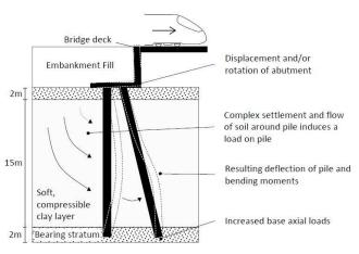
Figure 2. Geotechnical challenges facing a foundation engineer
