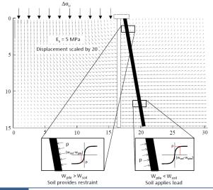
Figure 4. Ground movement immediately after embankment loading
