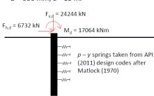
Bending moment per pile within from bridge loads:
