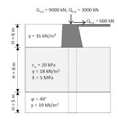
Factored Loads (EC 7 DA1/1 – A1 + R1 + M1):  $\gamma_G = [1.35, 1.0]; \, \gamma_Q = [1.5, 0] \\ F_{\nu,d} = 24244 \; kN; \, F_{h,d} = 6732 \; kN; \; M = 17064 \\ kNm$
