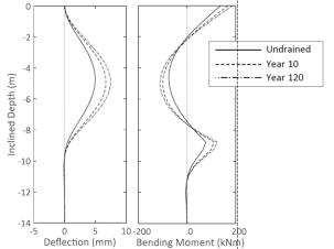
Figure 6. Additional bending from ongoing consolidation
