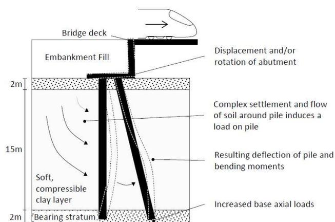
Figure 2. Geotechnical challenges facing a foundation engineer
