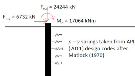
Bending moment per pile within from bridge loads:
